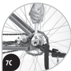
Remove rear wheel bolt. Attach quick release mounting bolt to the wheel. Re-tighten rear wheel bolt. Attach quick release pin to the trailer arm and latch securely. Figure 7A, 7B and 7C.
