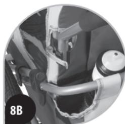
Remove the conversion kit wheel and handle bar before towing the trailer. The wheel can catch on the ground and the handle bar can hook onto things unexpectedly while turning.
