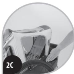
Unfold trailer canopy and close side locking clamps. Figure **2A**, **2B** and **2C**.
